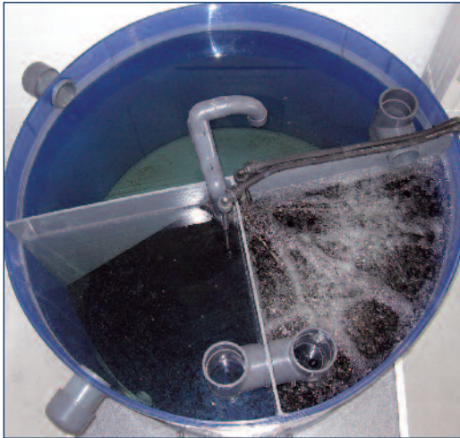
Top view AquaTop during aeration in the demonstration tank
